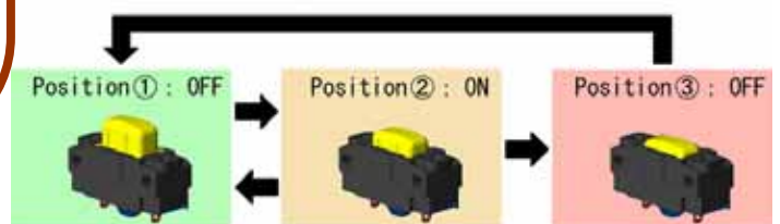
(b) Movement of 3 Position Switch
